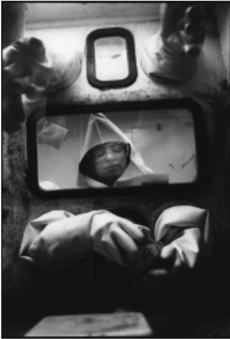
A glovebox for handling plutonium is a sealed environment kept under negative pressure and, when necessary, filled with inert gas to keep the plutonium inside it from igniting in the air. Safety procedures require this worker at the Plutonium Finishing Plant at the US Hanford site to wear anti-contamination clothing and to handle plutonium through the rubber gloves attached to the box.
